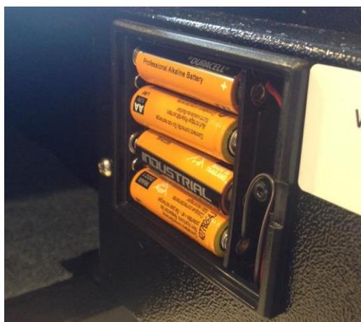
Change the batteries. Use a good quality AA battery, type LR6, alkaline.
