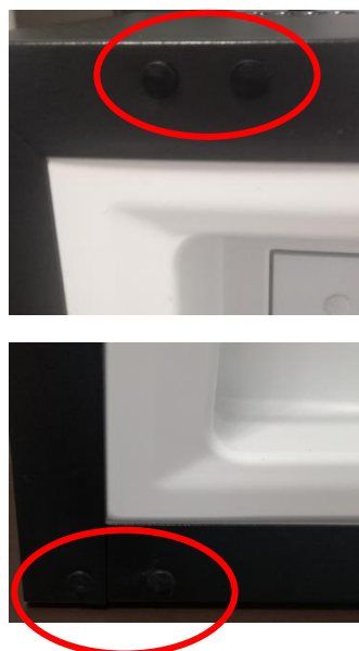
Remove the upper and lower left side plastic caps
